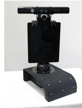
Fig. 1. Desktop telepresence robot prototype with tablet and Kinect.
