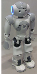
(a) NAO humanoid robot: 21 rotational joints; LEDs in the eyes; speakers in the ears; text-to-speech.
