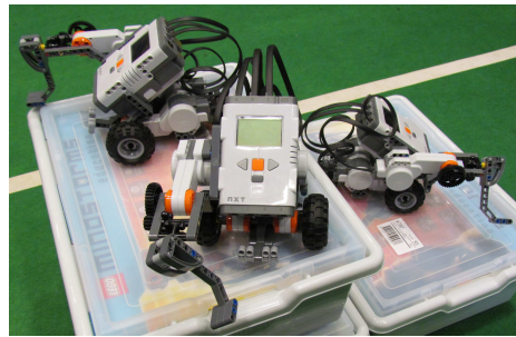
(b) Lego Mindstorms NXT robot: Two motors for the wheels; one motor for the arm; XBee communication module; internal speaker.
