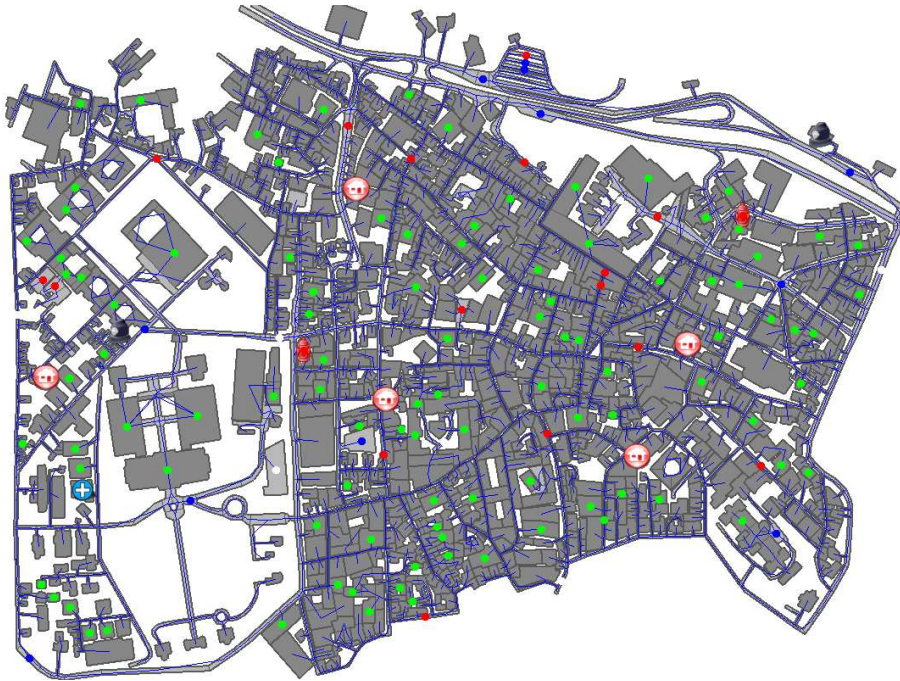
Figure 7.3: Screenshot of the RoboCup Rescue simulator showing the initial positions of the simulated robots. Green, red, blue, and white circles are civilians, fire engines, police cars, and ambulances respectively. The grey areas indicate buildings that darken as they burn down.
